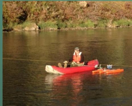
Acoustic Doppler Current Profiler – Towed Boat
