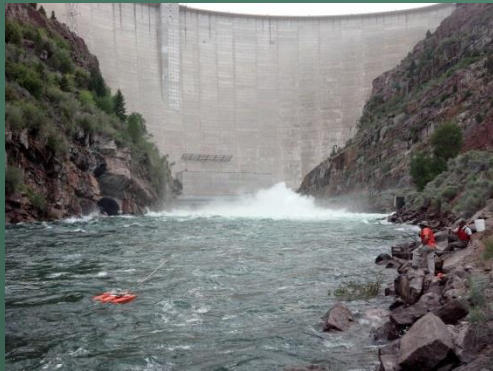
Acoustic Doppler Current Profiler – Bank Cableway
